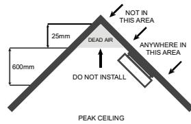
These alarms should be installed no more than 600mm vertically below the apex of a pitched ceiling. Where the depth from apex to eaves is 600mm or less the ceiling should be treated as flat.
