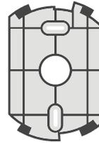
6. Align the baseplate to the plastic rawl plugs and fix in place using the provided screws.
